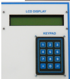
Student Response and Local Fault Insertion Panel
